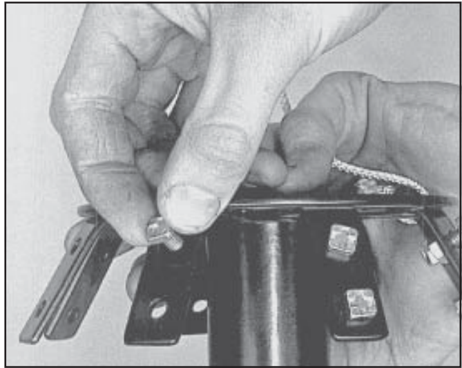
2.1 Pre-fit alloy nuts and bolts to the hub. Square heads face outwards. Leave the nuts slack.
