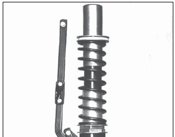
1.5 Wipe off surplus grease, then fit spring & thrust washer. (See also Fig A2, p11).
