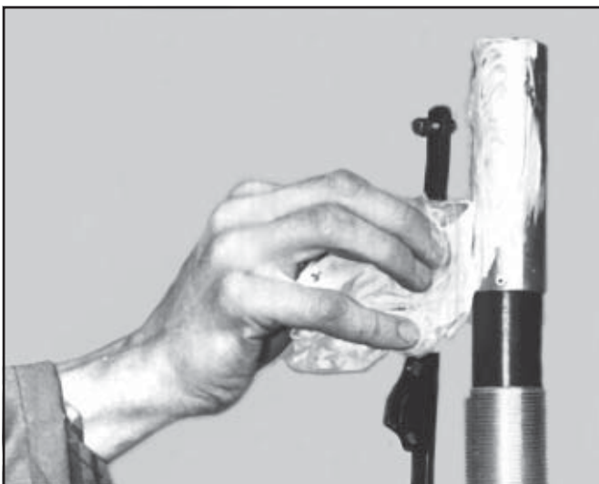
1.4 Apply waterproof grease from the sachet to the bush.
